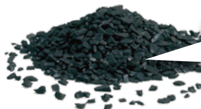
Granular activated carbon (4~6mmφ)
