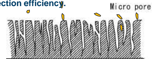
Can make uniform pore size artificially (10~20 Å)
