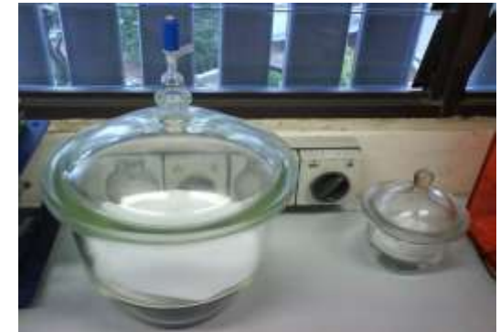
Methyl iodine static adsorption in desiccator (Type-K: Adsorption media test)
